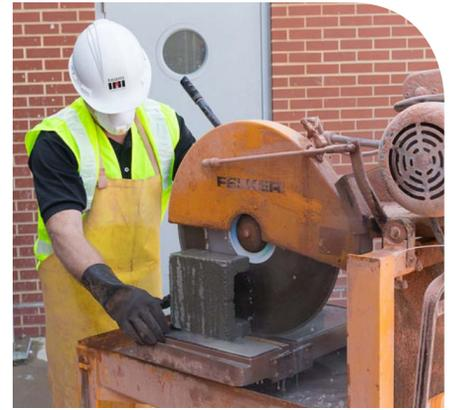
*Wetting process involves using water or a foam to keep dust down and out of the air.*
